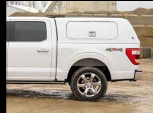
100SCC with optional flush side painted access doors for easy reach and a streamlined appearance.
